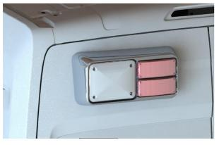
Application: Driver Side, High Roof, Rear Light Housing: Single 900 7 x 9 Light and two 700 Scene, LED or Halogen 3 x 7 Lights (2015 Ford Transit Cargo Van). Finish: polished exterior.
